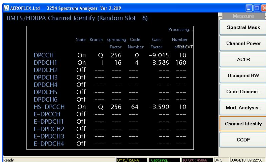
Fig. 13 Result of measuring Channel Identify for UMTS/HSUPA signal
